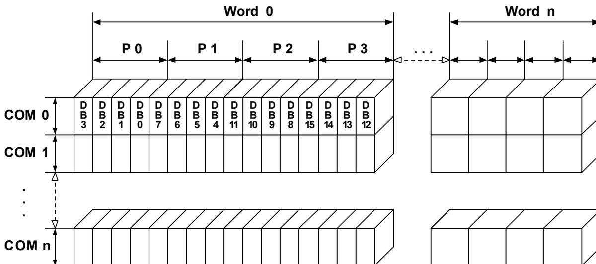
The delineation above shows the relation between the display memory and the SEG and COM lines of the LCD.
