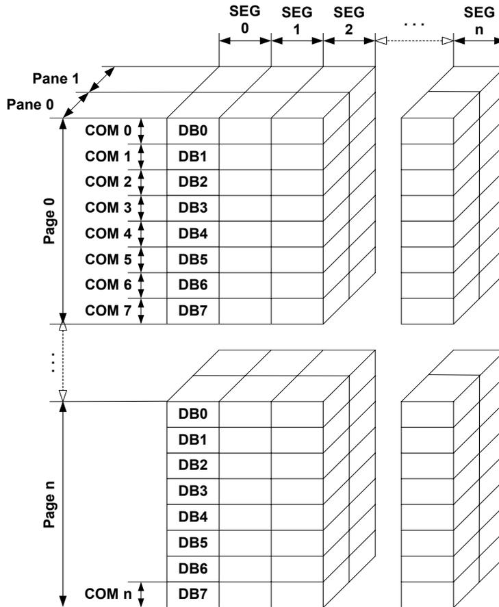
The picture above shows the relation between the display memory and the SEG and COM lines of the display. The display memory is divided into two panes for each pixel. The lower bit of each pixel is stored in pane 0 and the higher bit is stored in pane 1.
