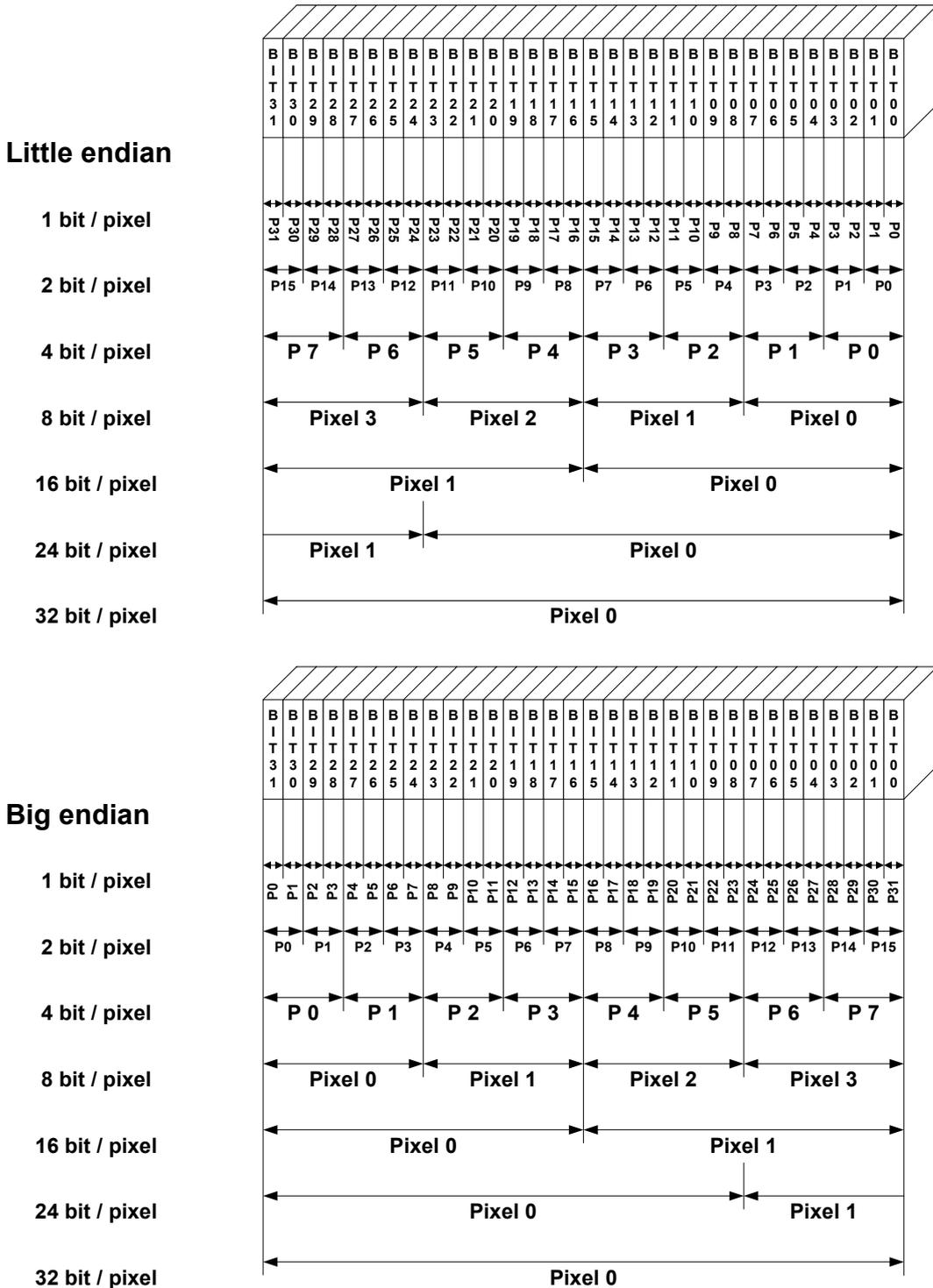
The picture above shows the relation between the display memory and the pixels of the LCD in terms of the color depth and the endian mode.
