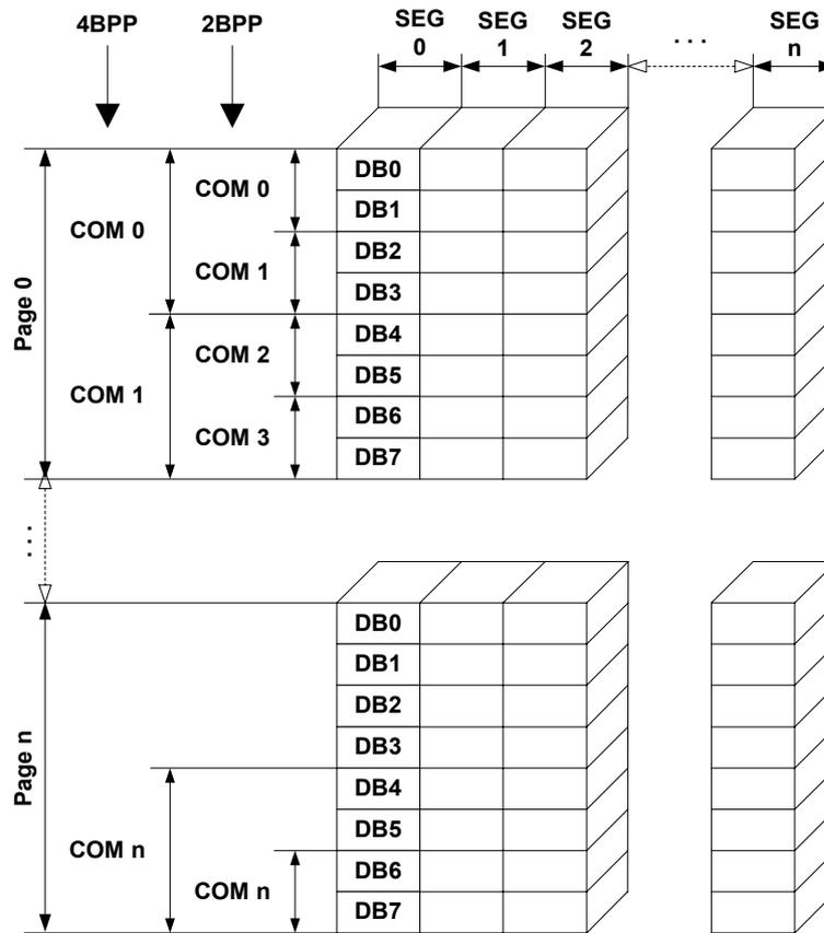
The picture above shows the relation between the display memory and the SEG and COM lines of the display.
