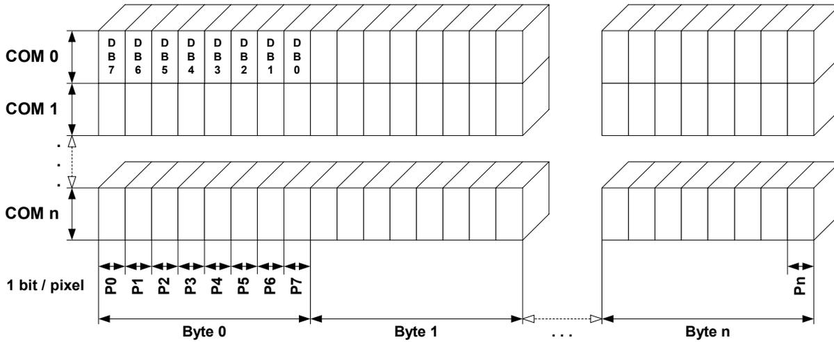
The picture above shows the relation between the display memory and the SEG and COM lines of the LCD.
