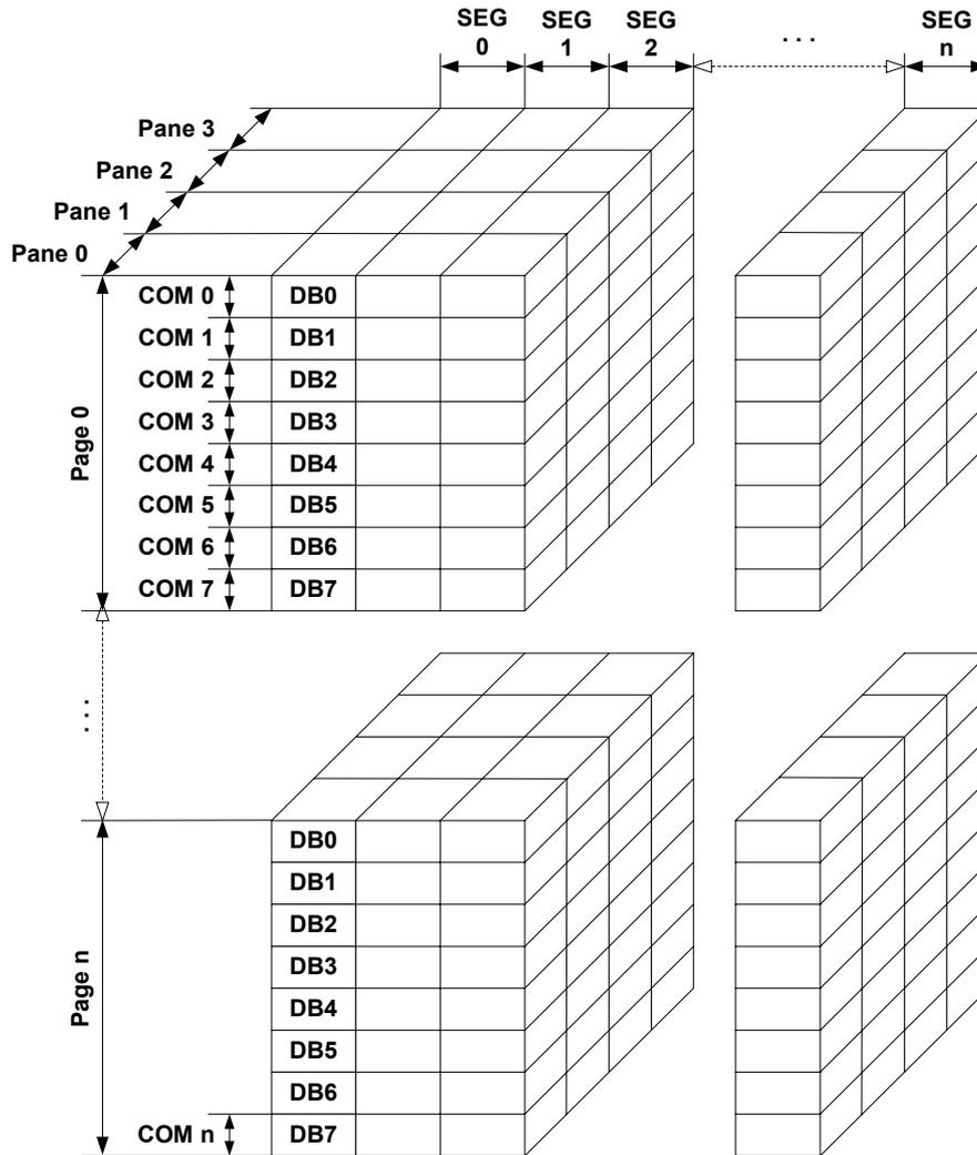
The picture above shows the relation between the display memory and the SEG and COM lines of the LCD. The display memory is divided into four panes for each pixel. The least significant bit (LSB) of each pixel is stored in pane 0 and the MSB is stored in pane 3.
