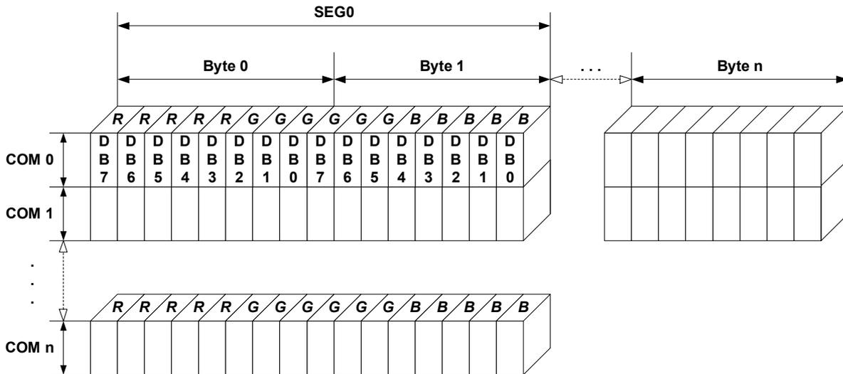
The picture above shows the relation between the display memory and the SEG and COM lines of the display.
