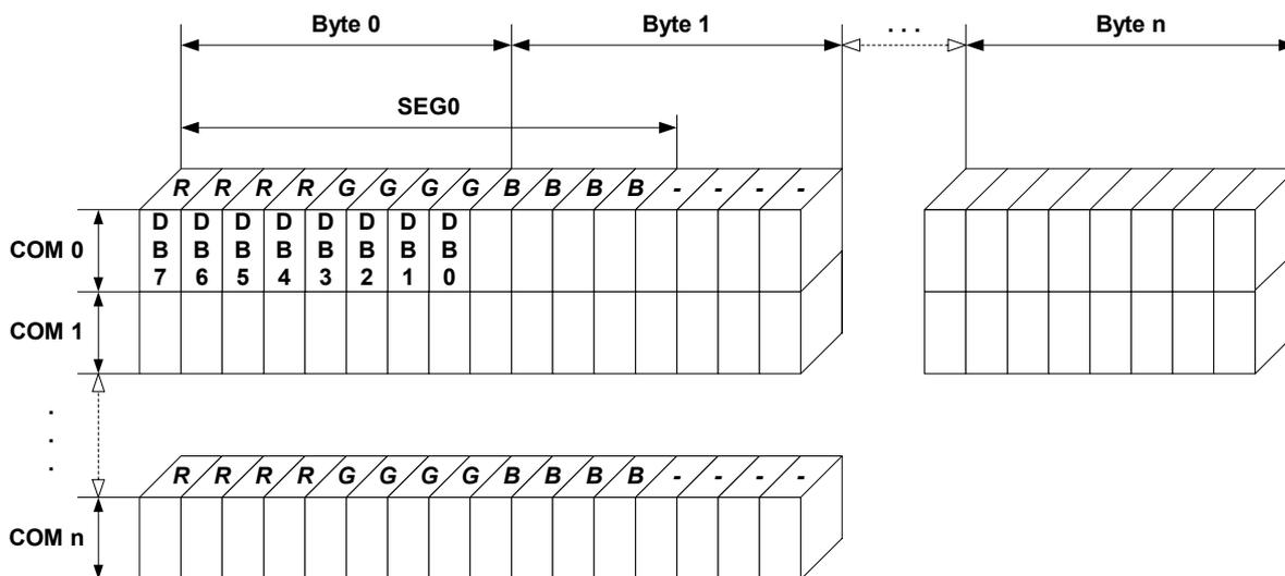
The picture above shows the relation between the display memory and the SEG and COM lines of the LCD.
