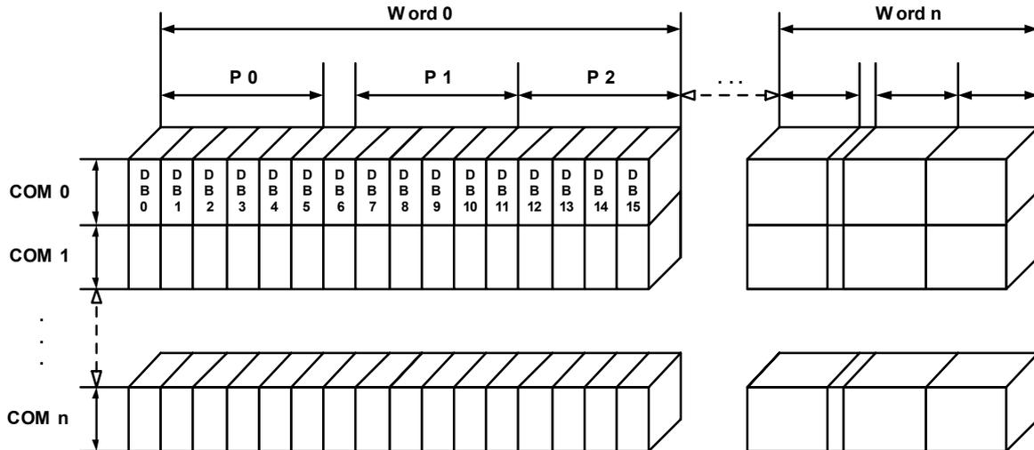
The picture above shows the relation between the display memory and the pixels of the LCD in terms of the color depth
