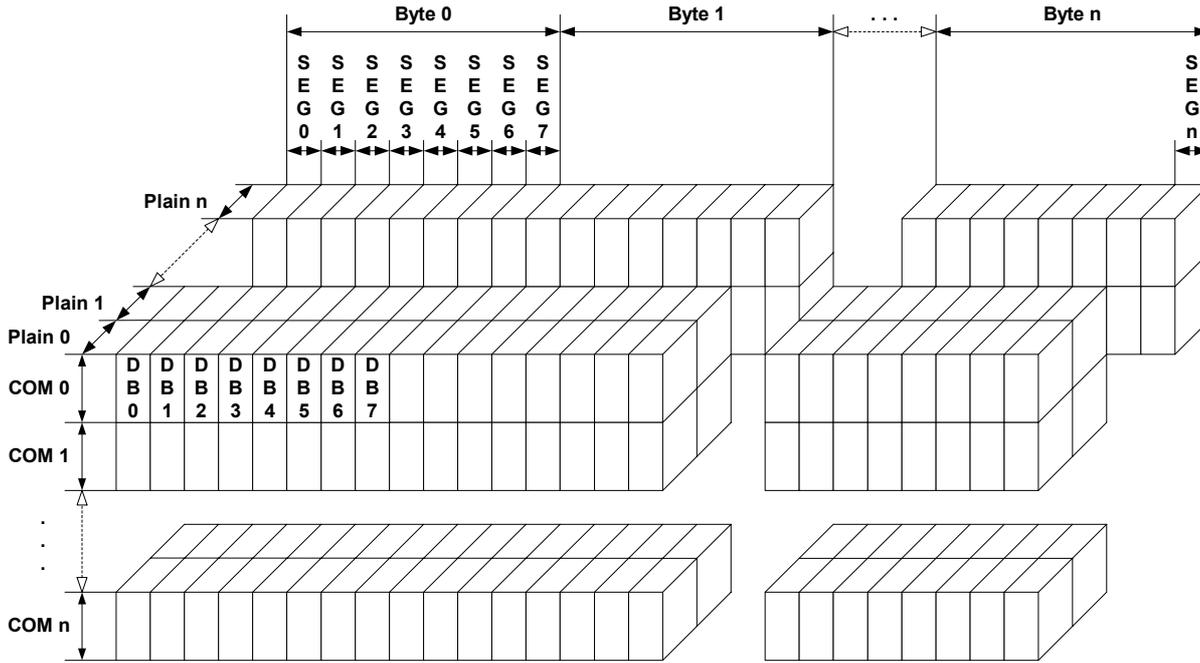
The picture above shows the relation between the display memory and the SEG and COM lines of the display. The display memory is divided into separate plains for each bit of the colors. This means that bit 0 of each pixel is stored in plain 0, the bit 1 in plain 1 and so on. The advantage of this method is that each color bit of the display data can be accessed very quickly.
