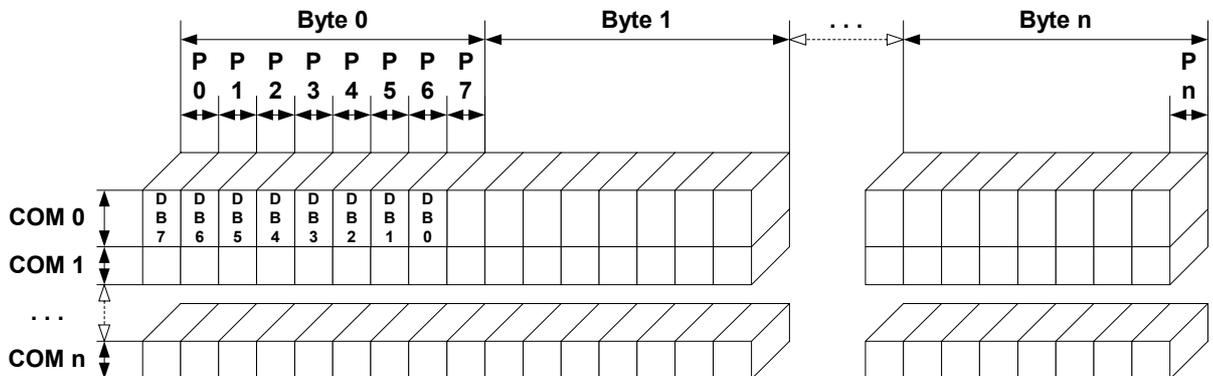
The picture above shows the relation between the display memory and the SEG and COM lines of the LCD.
