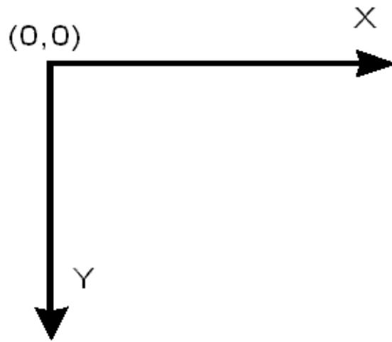
X-values are always to the right; positive Y-values are always down. The above graph illustrates the coordinate system and directions of the X- and Y- axes. All coordinates passed to an API function are always specified in pixels.
